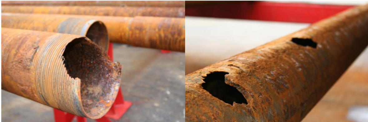
Figure 43 Corroded tubing due to incompatibility between the tubing material and injection water quality
